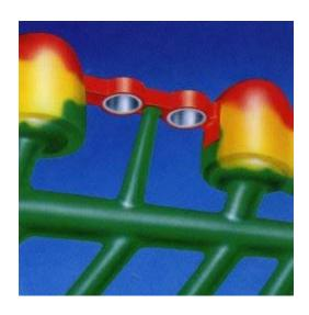
Use casting sprues with a diameter of 3mm on the female parts.
