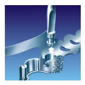
After casting remove the threaded core, useed as a spacer. However the nut should be covered with wax during electrolytic polishing, in order to avoid damage. Finish as usual.
