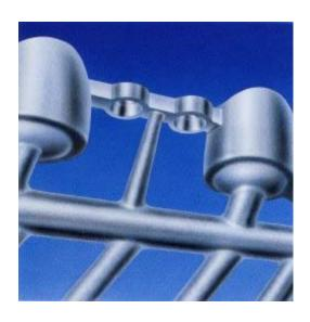
When using bars it is also important to position an extra casting sprue in the middle to obtain an optimal result.
