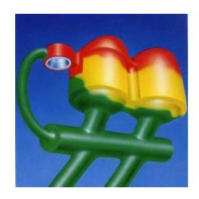
It is important to use an extra casting sprue on one-bar eyelets to obtain an optimal result.
