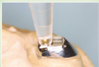
Using the tool, check the fit of the cast cap by inserting the sphere into the base.
